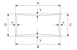
Right/left distortion = (4x)/(A + B)Up/down distortion = (4y)/(C + D)
